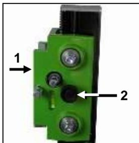
To unlock the carriage (1) pull out the lock knob (2).
