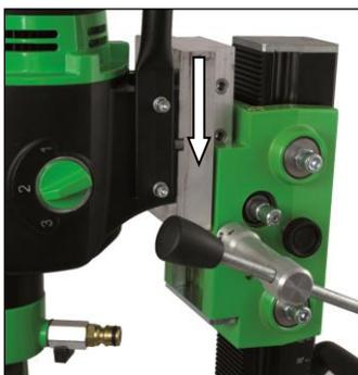
The mounting plate is put on in such a way with the fitting key on the machine that the socket is in the mounting plate on the same side as the gear switch of the machine. Afterwards the four screws are insert and tightened firmly.
