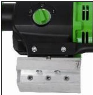
Move the machine holder upwards until it locks in the top position.
